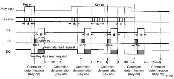
t5......Key scan execution time (25600T [s]) when the key data for two key scan operations matches.
