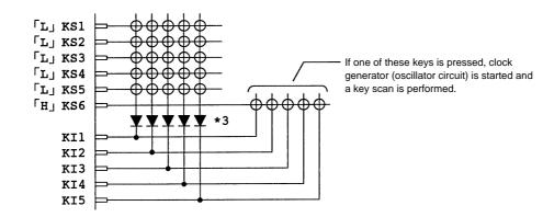
Note \*: These diodes are required to reliably recognize multiple key presses on the KS6 line when the IC is set to sleep mode with only KS6 set to high as in the example above. That is, they prevent incorrect recognition of key presses due to sneak currents arising from simultaneous presses of keys on the KS1 through KS5 lines.
