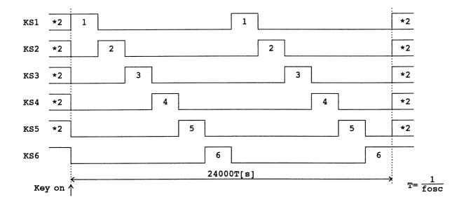
Note \*: The high-level and low-level states in sleep mode are set according to the control data S0 and S1. Key scan output signals are not output from pins set to the "L" state.
