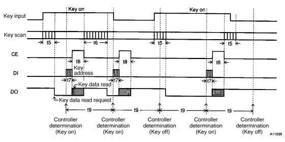
t5......Key scan execution time (25600T [s]) when the key data for two key scan operations matches.
