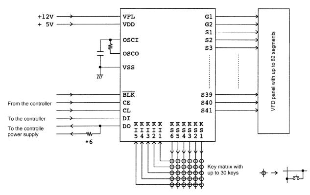
Note \*: Since DO is an open-drain output, a pull-up resistor is required. Select a value in the range 1 to 10 kΩ that is most appropriate for the capacitance of the external lines so that the waveform is not distorted.
