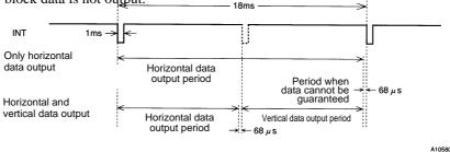
Figure 2 External Interface Basic Timing
