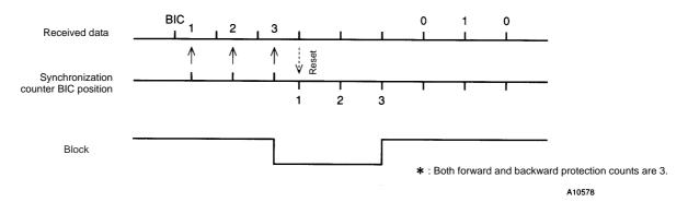
Figure 1 Block Synchronization Protection Operation (forward → backward → forward)
