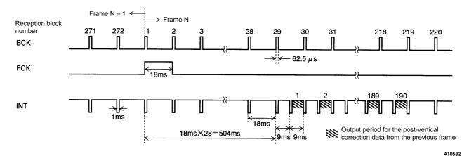
Figure 4 Post-Vertical Correction Data Output Timing
