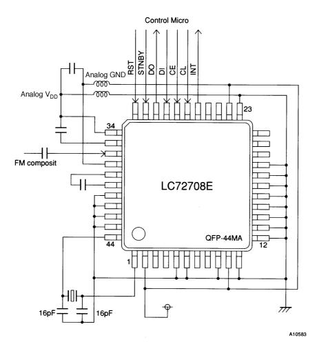
Caution: The value of the DO (pin 31) pull-up resistor must be chosen to be appropriate for the frequency of the transfer clock used.
