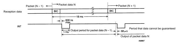
Figure 3 Timing of Data Reception and Block Synchronization Data Output
