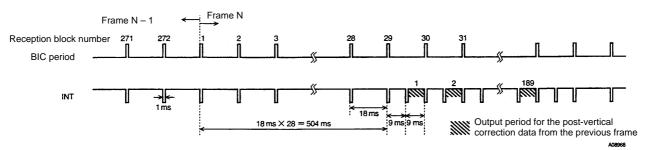
Figure 4 Vertical Correction Data Output Timing
