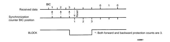
Figure 1 Block Synchronization Protection Operation (forward → backward → forward)
