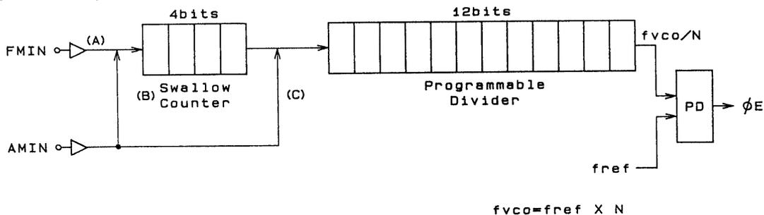
Figure 7 Programmable Divider
