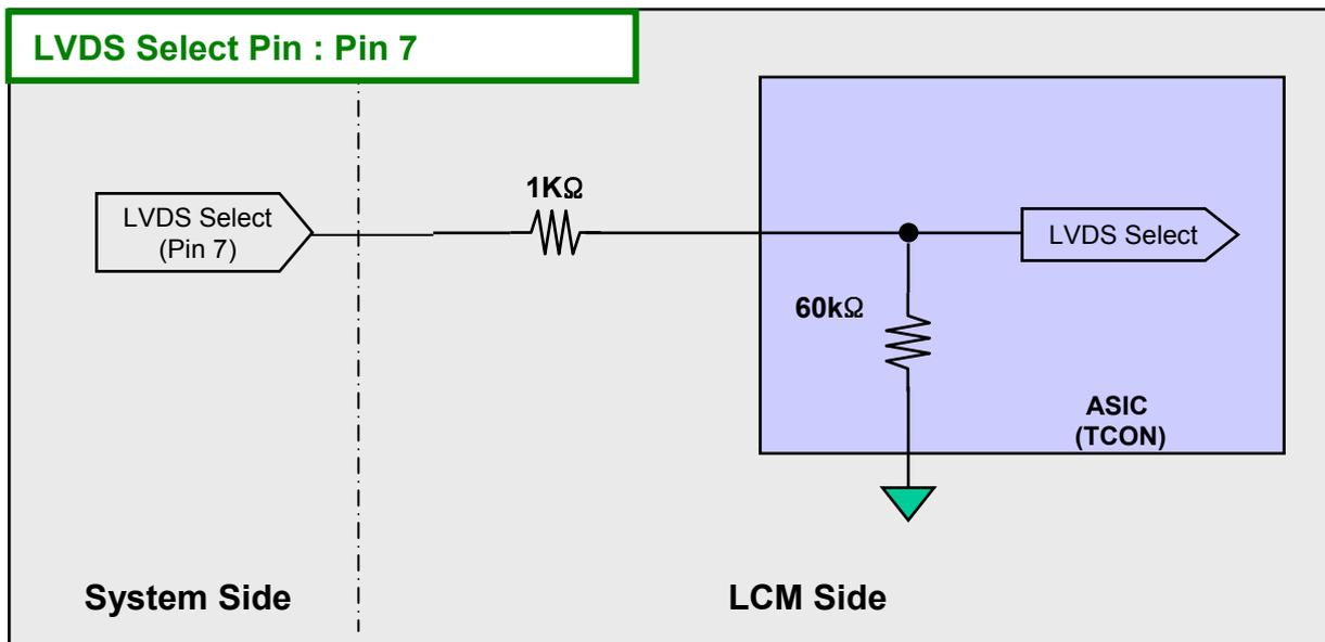
2) Circuit Block Diagram of Bit Selection pin
