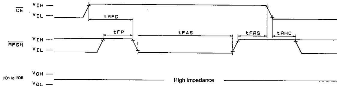
Note: CS,  $\overline{OE}$ ,  $\overline{WE}$ , A0 to A15: "H" or "L"
