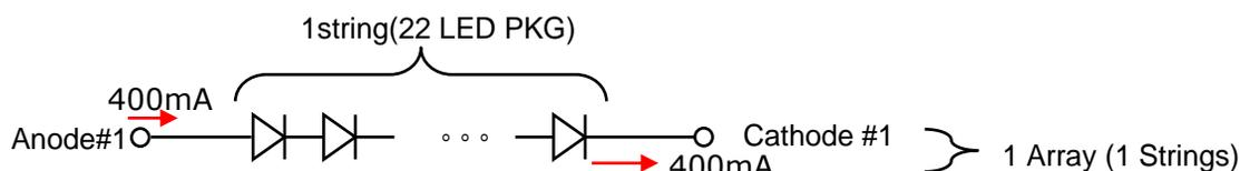
4. The forward voltage( $V_F$ ) of LED array depends on ambient temperature (Appendix-VII)
