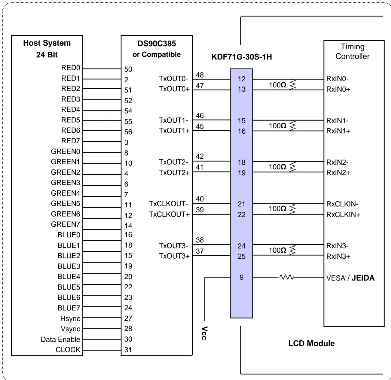
Note :1. The LCD module uses a 100 Ohm[Ω] resistor between positive and negative lines of each receiver input.
