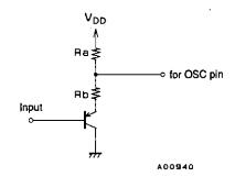
Use the LB1870  $V_{REG}$  output for the  $V_{DD} = 6.3 \text{ V}$  case.
