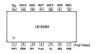
Note: Both GND pins must be grounded.
