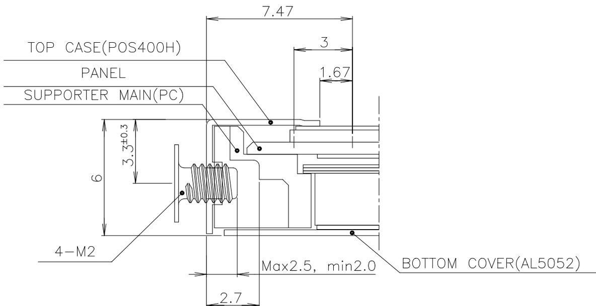
\*MOUNTING SCREW DEPTH : MAX 2.5mm
