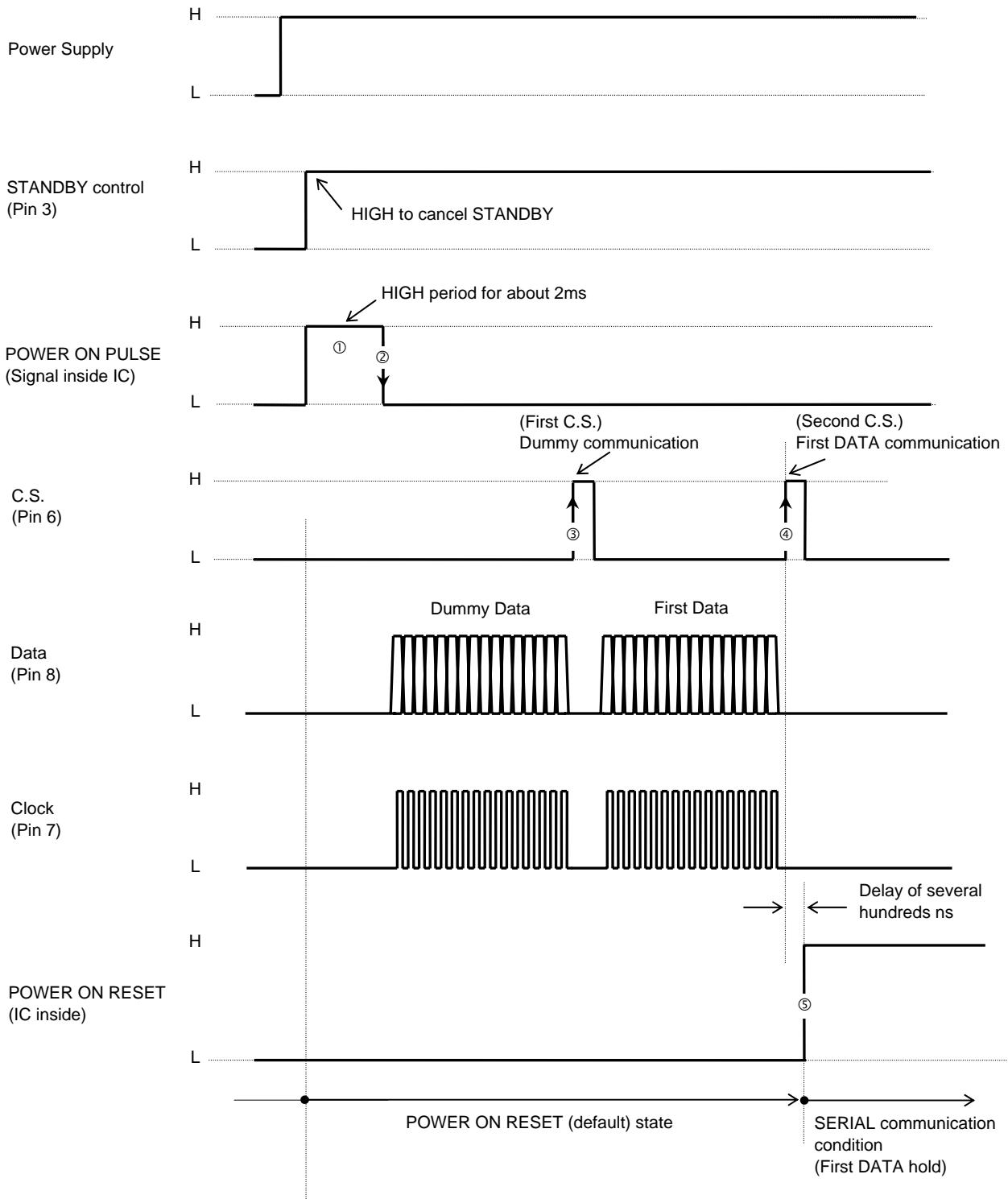
The POWER ON RESET state covers a period up to the rise ⑤ of the second C.S. input after fall ② of POWER ON PULSE ① generated inside IC when the power is supplied and the STANDBY control is canceled. ③ is the dummy communication.
