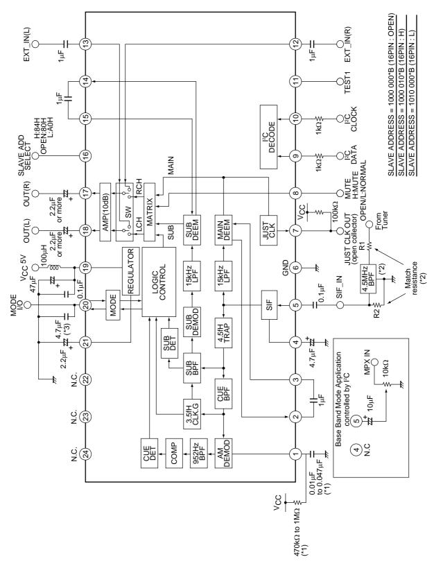
The value of  $(1^*)$ ,  $(2^*)$ , and  $(3^*)$  affects sensitivity for signal detection. It must be adjusted depending on the circumstances by the user.
