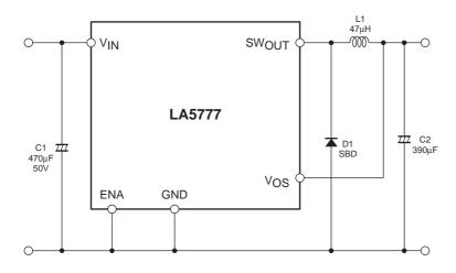
Note: ENA pin starts operation with LOW voltage input.
