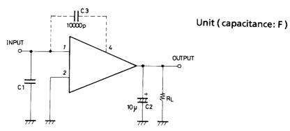
Note: Capacitor C3 is not required unless radio noise is a problem.
