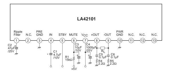
\* LA42101 employs the zero-bias type input circuit, with the input pin potential being nearly zero (about 0.01V). Accordingly, the polarity must be determined according to the DC potential of a circuit connected to the previous stage of LA42101.
