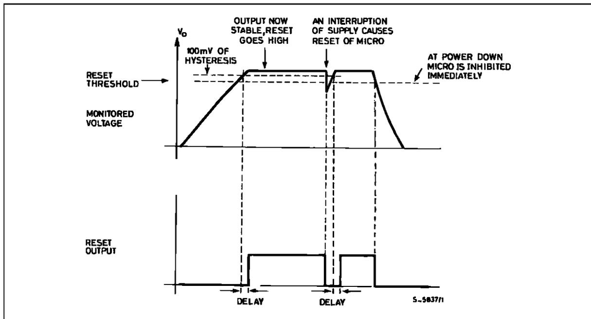
Figure 2 : Soft Start Waveforms
