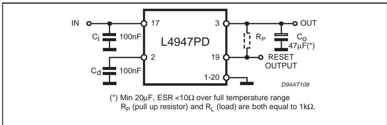
**ELECTRICAL CHARACTERISTICS** (refer to the test circuit,  $V_i = 14.4V$ ,  $C_o = 47\mu F$ ,  $ESR < 10\Omega$ ,  $R_p = 1K\Omega$ ,  $R_L = 1K\Omega$ ,  $-40^\circ C \leq T_J \leq 125^\circ C$ , unless otherwise specified)
