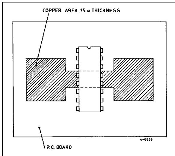
During soldering the pins temperature must not exceed  $260^{\circ}\text{C}$  and the soldering time must not be longer than 12 seconds.
