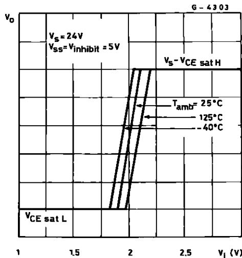
**Figure 7 :** Output Voltage versus Inhibit Voltage
