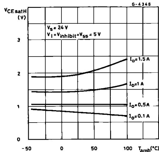
**Figure 4 :** Sink Saturation Voltage versus Ambient Temperature
