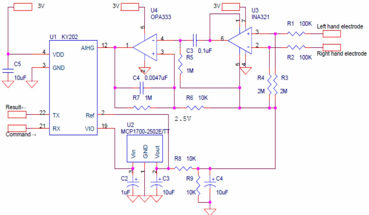
Data acquisition from analog input using internal amplifier
