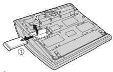
Match the polarity and snap the battery to the battery snap as shown.
