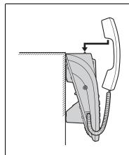
To temporarily set the handset down during a conversation, place it as shown here.
