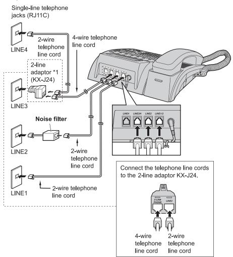
\*1 2-line adaptor merges a 2-wire (single line) telephone outlet with another 2-wire (single line) telephone line onto a single 4-wire (2-line) telephone line cord.
