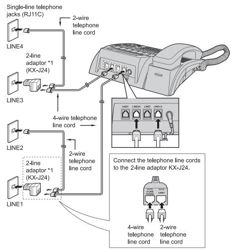
\*1 2-line adaptor merges a 2-wire (single line) telephone outlet with another 2-wire (single line) telephone line onto a single 4-wire (2-line) telephone line cord.
