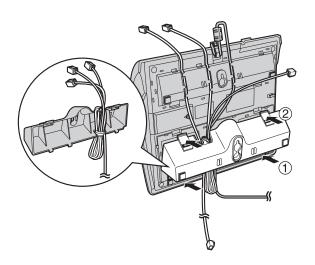
**4** Connect the telephone line cord. Mount the unit, then slide down.
