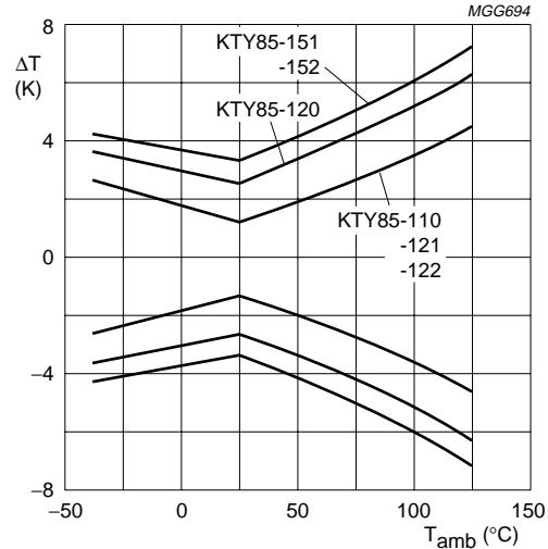
Fig.2 Maximum expected temperature error ( $\Delta T$ ).
