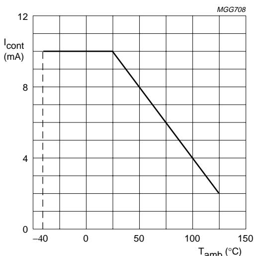
Fig.5 Maximum operating current for safe operation.
