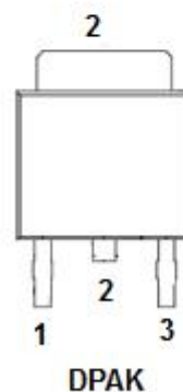
PIN : 1 Base 2 Collector 3 Emitter TO-252 Package
