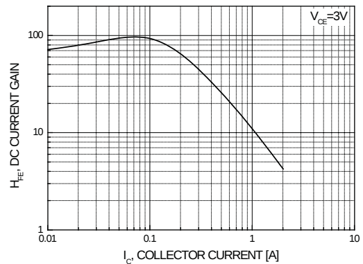
Figure 2. DC Current Gain
