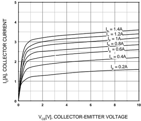
Figure 1. Static Characteristic
