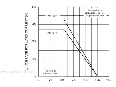
$T_{\rm C}$ , CASE TEMPERATURE (°C) Fig. 1 Forward. Current Derating Curve
