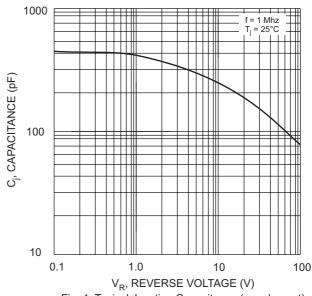
Fig. 4 Typical Junction Capacitance (per element)
