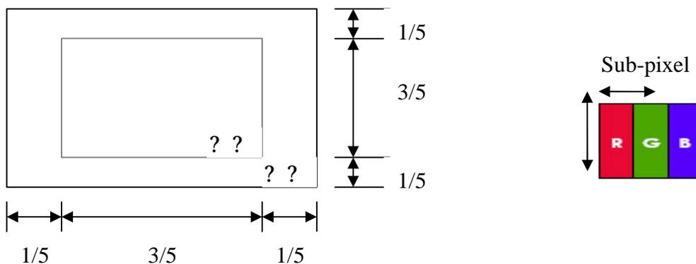
Note: 1. Dot defect is defined as the defective area of the dot area is larger than 50% of the dot area . And the bright dot defect must be visible through 5% ND filter.
