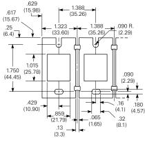
37D633 will mount eight 27E488 sockets in one length of aluminum strip mea-suring 10.97" x 2.25" x .062". (278.64 x 57.15 x 1.57)
