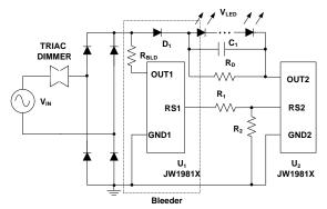
TRIAC Dimming can be achieved if two chips are used.  $R_{BLD}$ =3.3 $K\Omega$  is recommended to decrease the power loss of the  $U_1$ .  $D_1$  is not essential if  $C_1$  is not connected.  $R_2$  is used to set the LED current ( $I_{LED}$ ). If the instantaneous input voltage is lower than the LEDs' VF ( $V_{LED}$ ) when the TRIAC is on, the approximate value of  $I_{LED}$  is:
