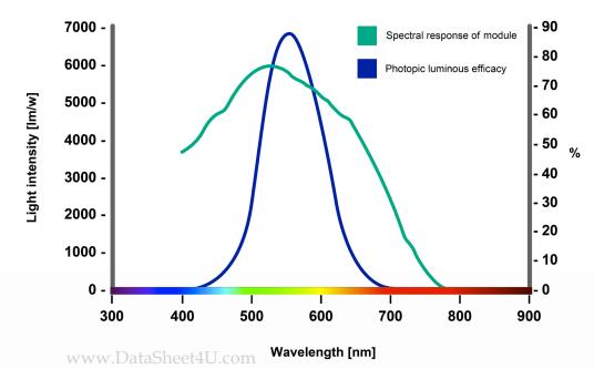
G24i's dye sensitised indoor photovoltaic modules have been optimised to work under indoor lighting providing the highest power density.
