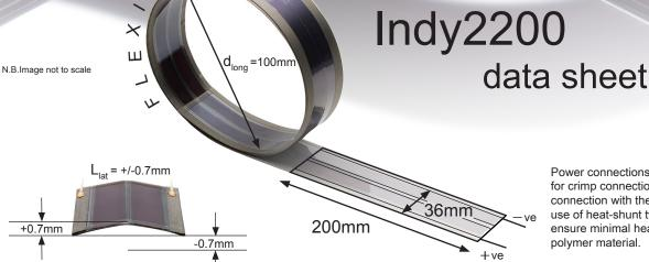
Power connections are suitable for crimp connection or soldered connection with the appropriate use of heat-shunt tweezers to ensure minimal heating of the polymer material.
