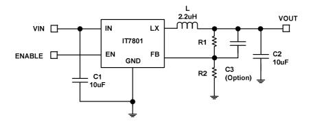
**Figure 1. Typical Application Circuit**
