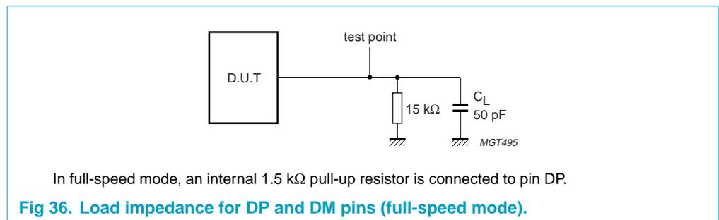
In full-speed mode, an internal 1.5 kΩ pull-up resistor is connected to pin DP.
