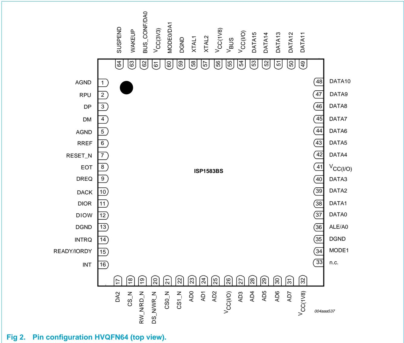
Fig 2. Pin configuration HVQFN64 (top view).
