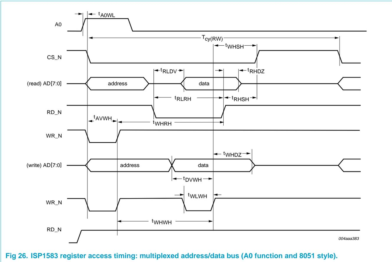
Fig 26. ISP1583 register access timing: multiplexed address/data bus (A0 function and 8051 style).
