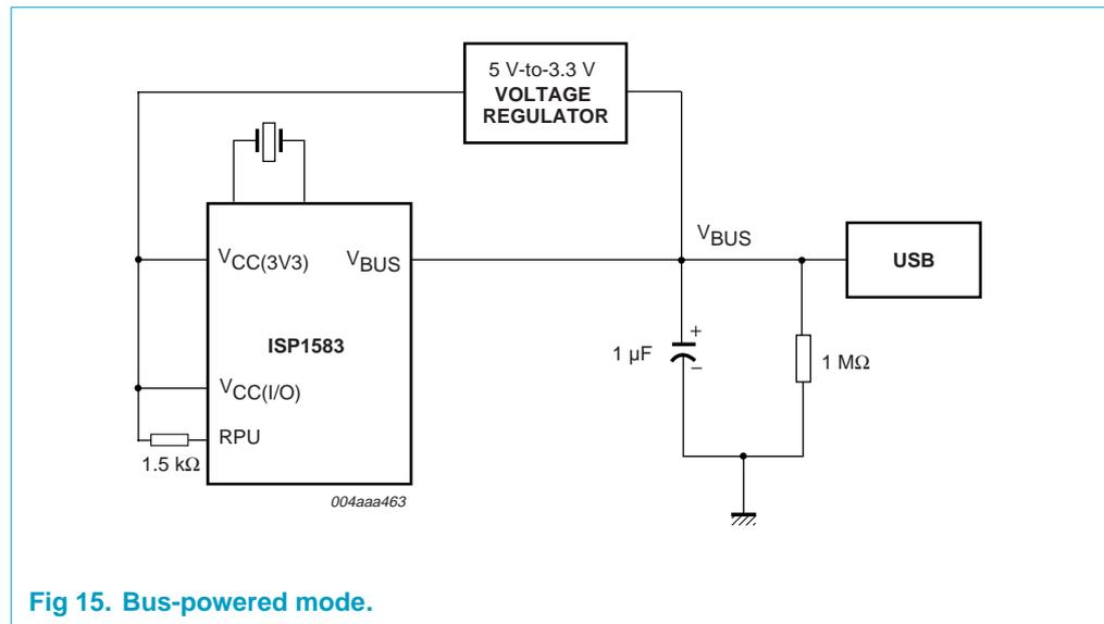
Fig 15. Bus-powered mode.
