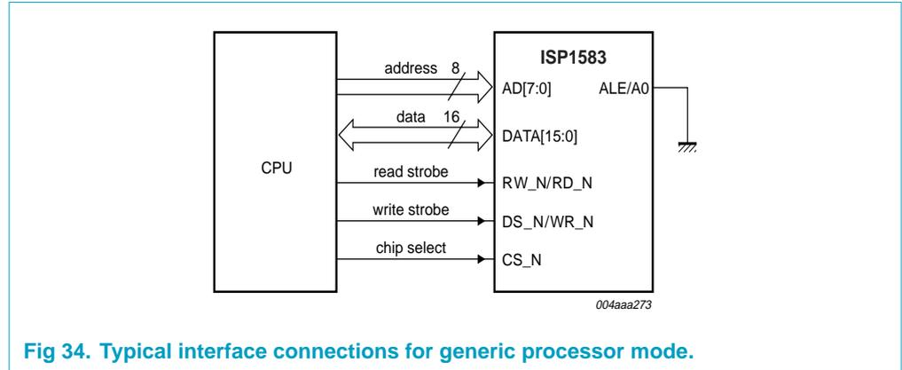
Fig 34. Typical interface connections for generic processor mode.
