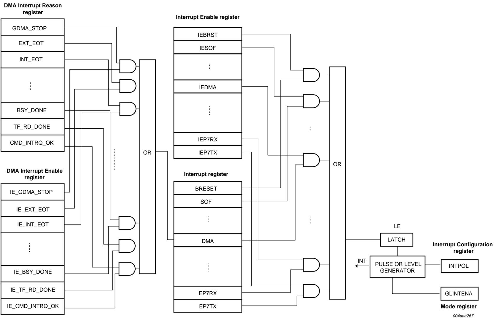
Fig 4. Interrupt logic.
