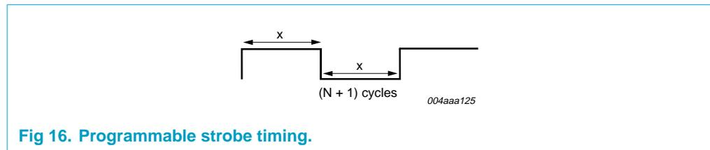
**Fig 16. Programmable strobe timing.**
