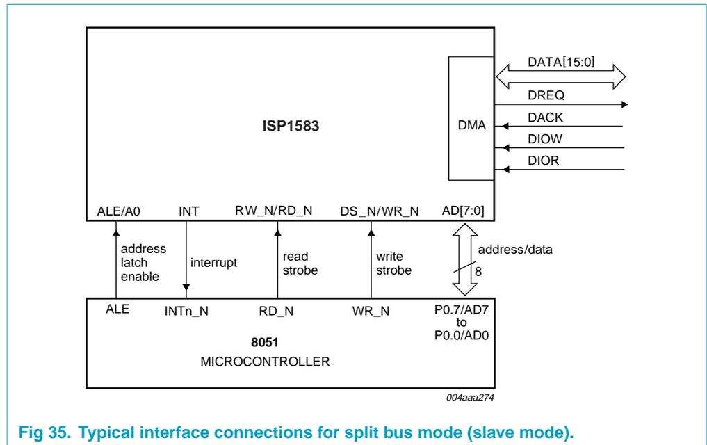
Fig 35. Typical interface connections for split bus mode (slave mode).
