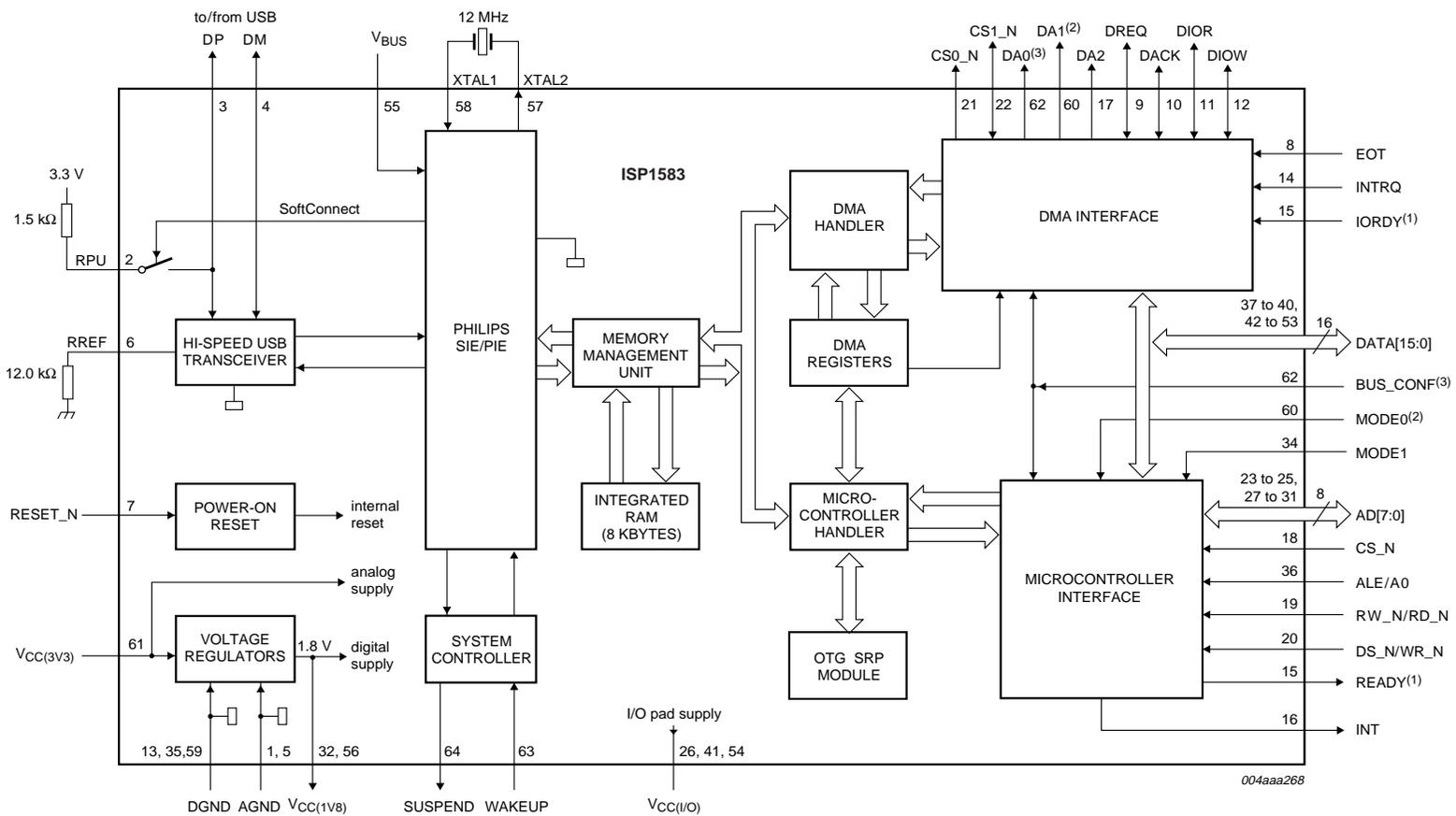
The direction of pins DREQ, DACK, DIOR and DIOW is determined by bit MASTER (DMA Hardware register) and bit ATA\_MODE (DMA Configuration register).
