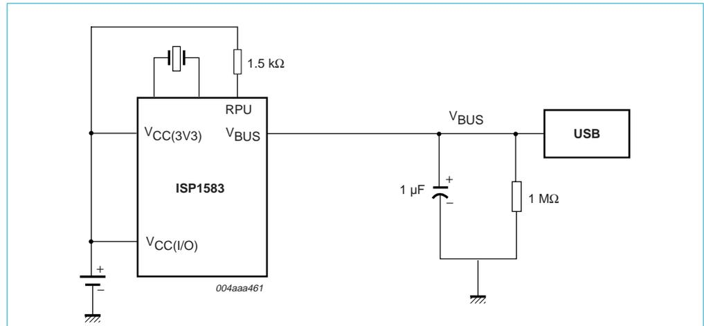
Fig 14. Self-powered mode.
