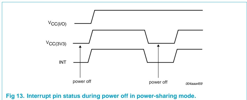
Fig 13. Interrupt pin status during power off in power-sharing mode.
