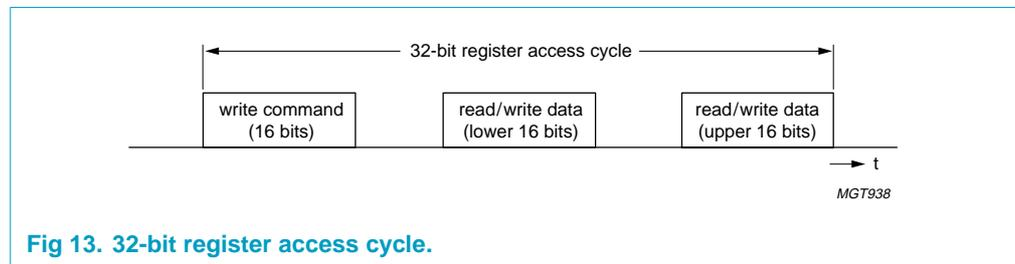
Fig 13. 32-bit register access cycle.
