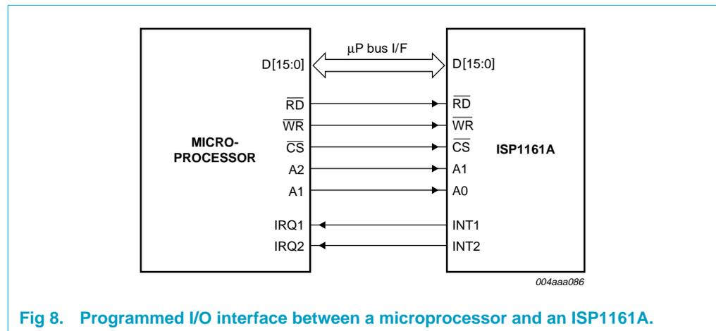
Fig 8. Programmed I/O interface between a microprocessor and an ISP1161A.
