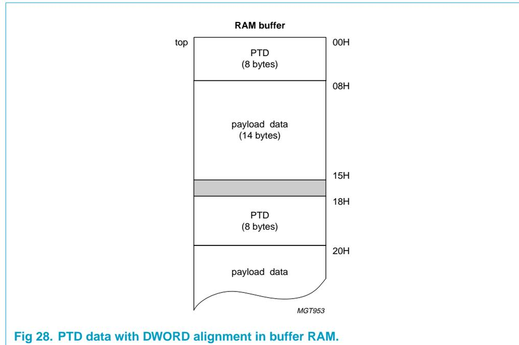
Fig 28. PTD data with DWORD alignment in buffer RAM.
