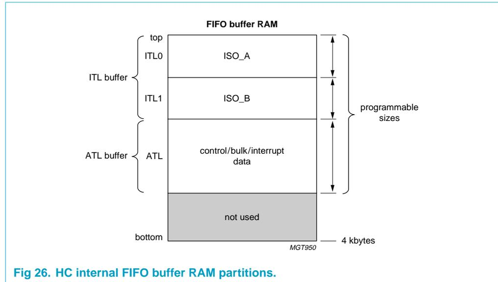
**Fig 26. HC internal FIFO buffer RAM partitions.**
