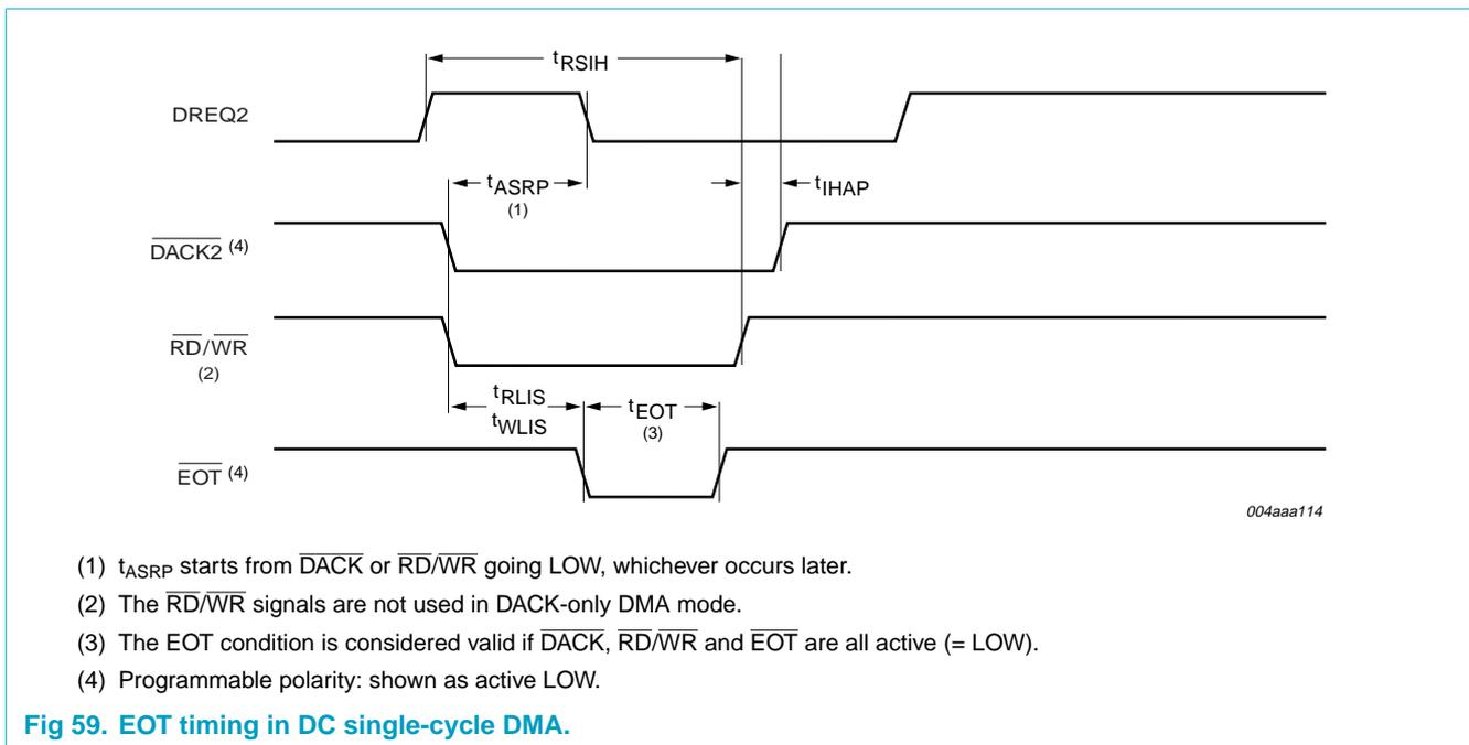
Fig 59. EOT timing in DC single-cycle DMA.
