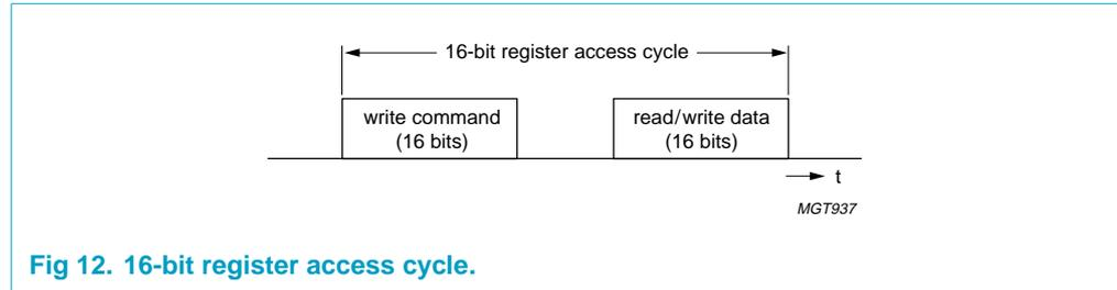
Fig 12. 16-bit register access cycle.
