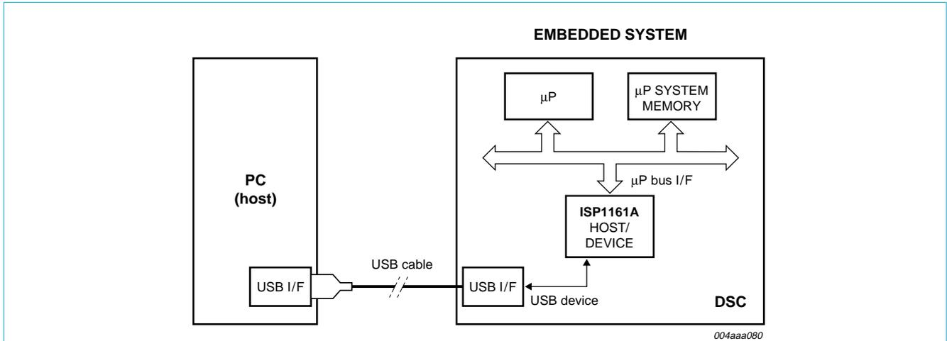
Fig 1. ISP1161A operating as a USB device.
