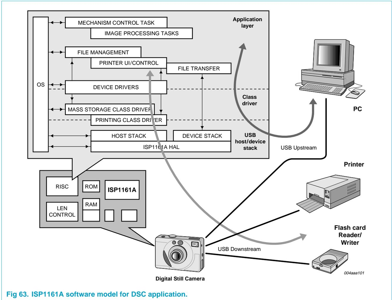
Fig 63. ISP1161A software model for DSC application.
