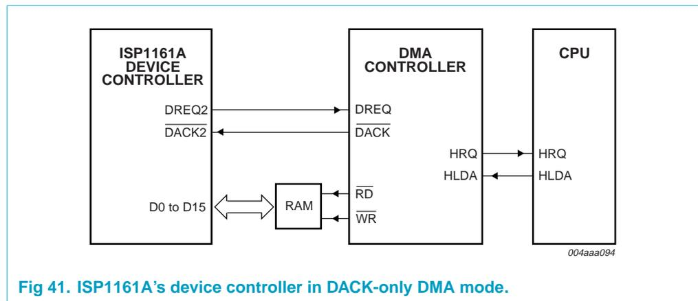
Fig 41. ISP1161A's device controller in DACK-only DMA mode.
