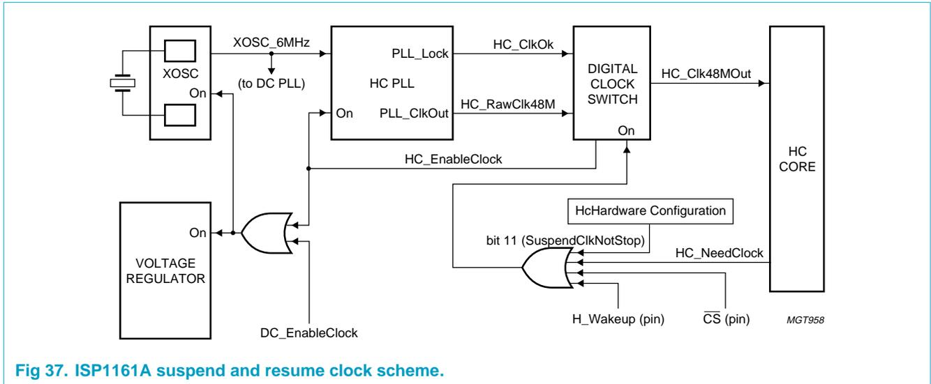
Fig 37. ISP1161A suspend and resume clock scheme.
