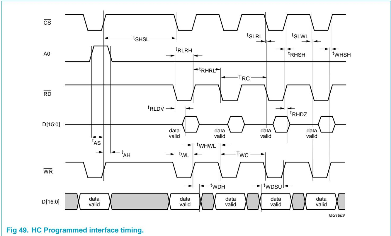
Fig 49. HC Programmed interface timing.
