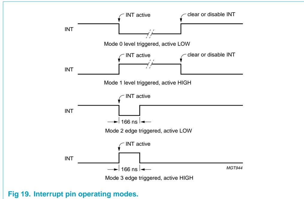
Fig 19. Interrupt pin operating modes.
