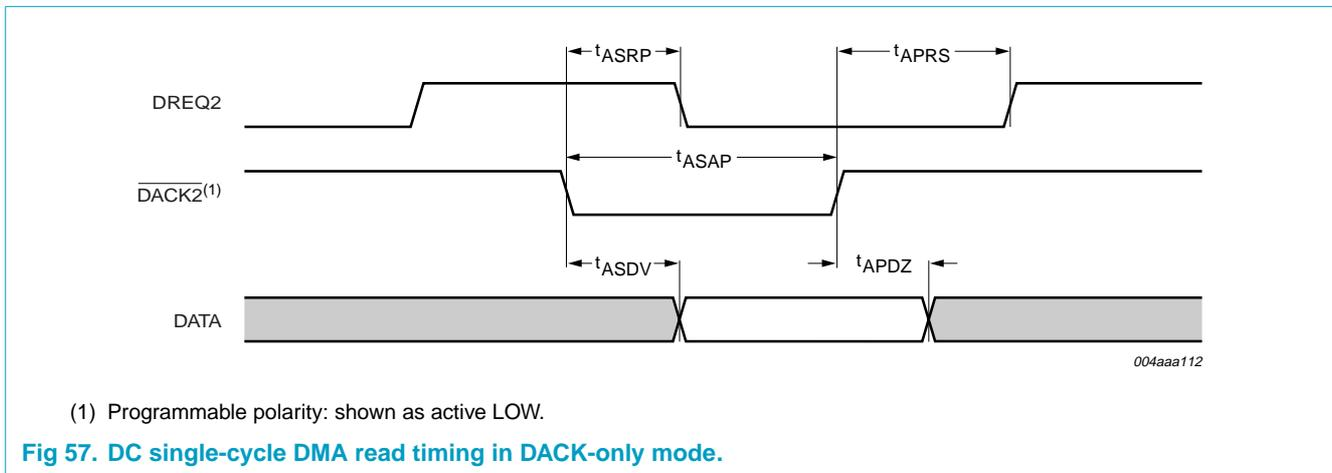
Fig 57. DC single-cycle DMA read timing in DACK-only mode.
