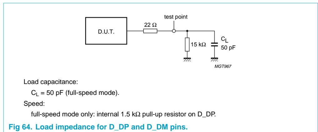
Fig 64. Load impedance for D\_DP and D\_DM pins.
