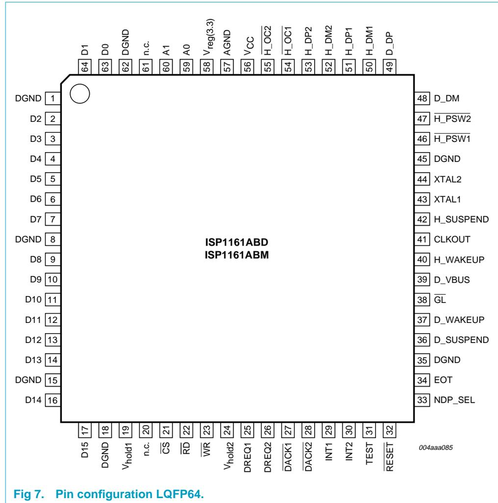
Fig 7. Pin configuration LQFP64.
