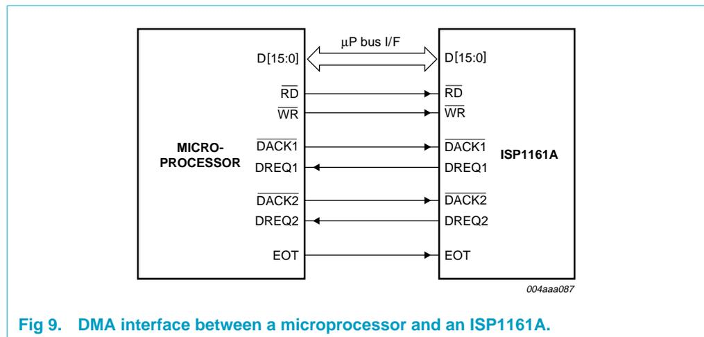
Fig 9. DMA interface between a microprocessor and an ISP1161A.
