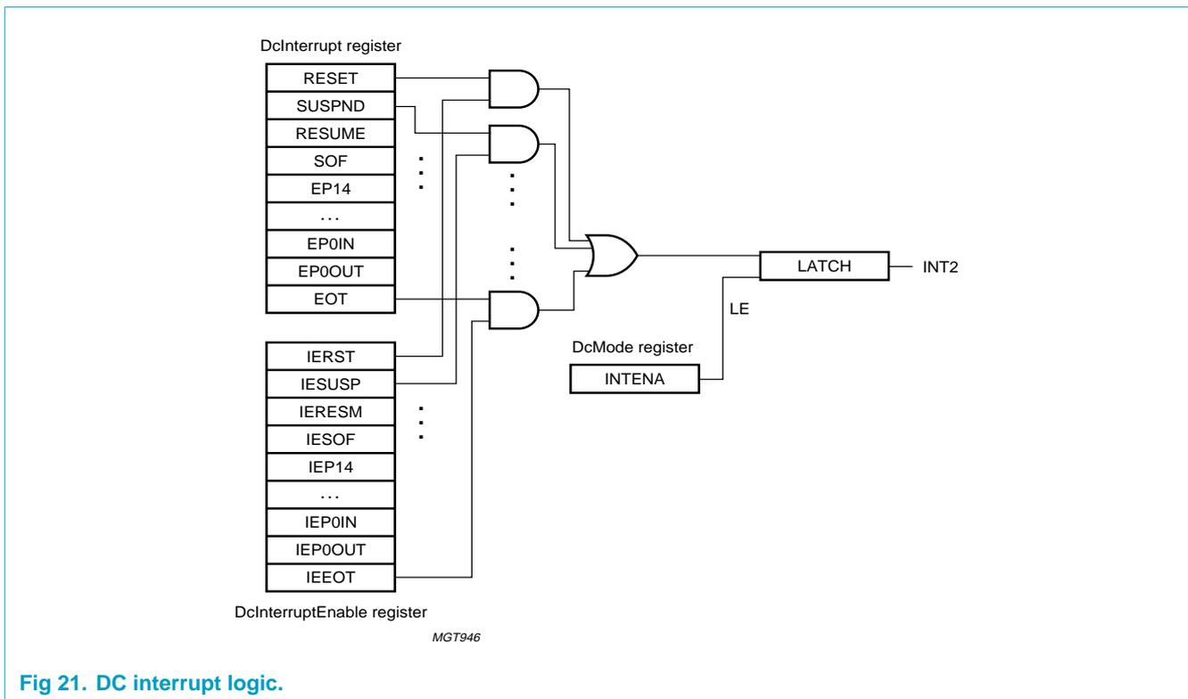
Fig 21. DC interrupt logic.
