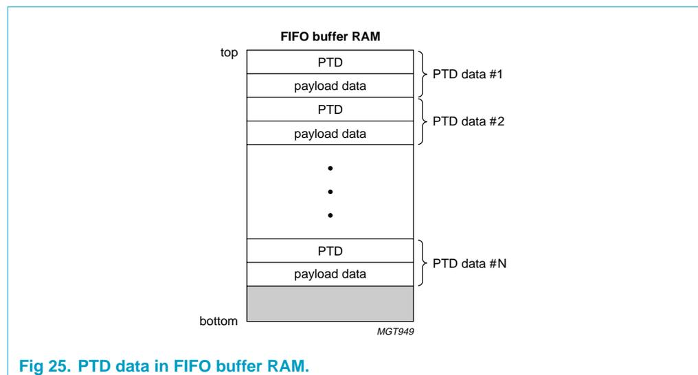
**Fig 25. PTD data in FIFO buffer RAM.**
