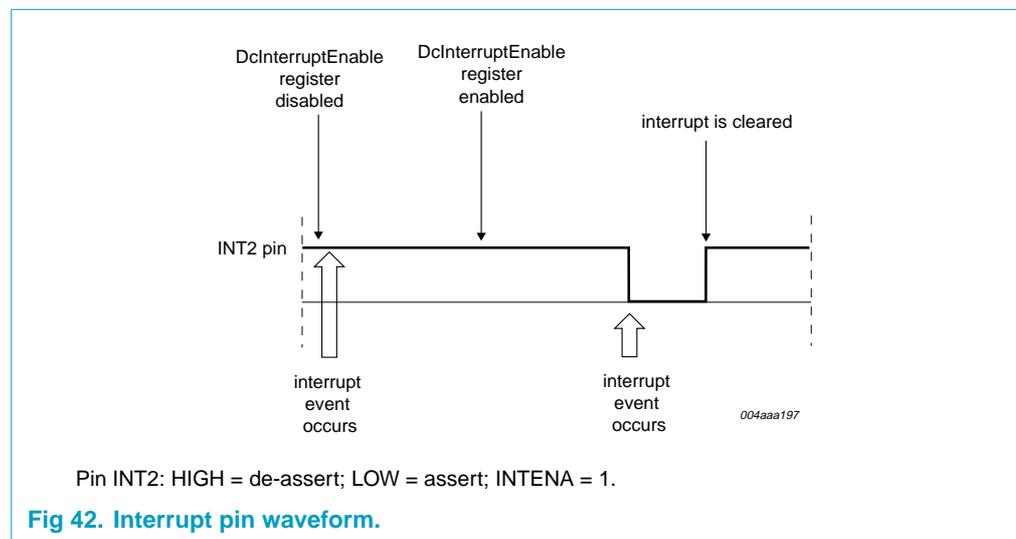
Fig 42. Interrupt pin waveform.
