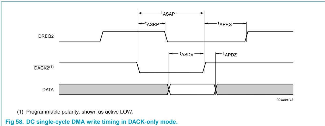
Fig 58. DC single-cycle DMA write timing in DACK-only mode.
