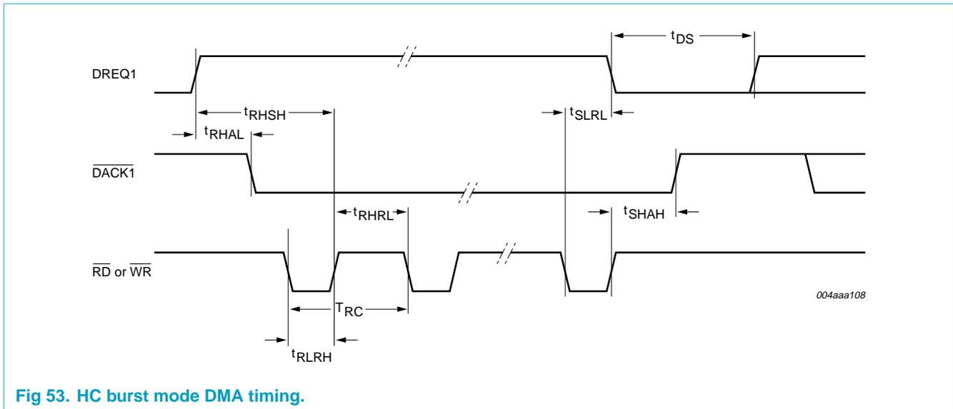
Fig 53. HC burst mode DMA timing.
