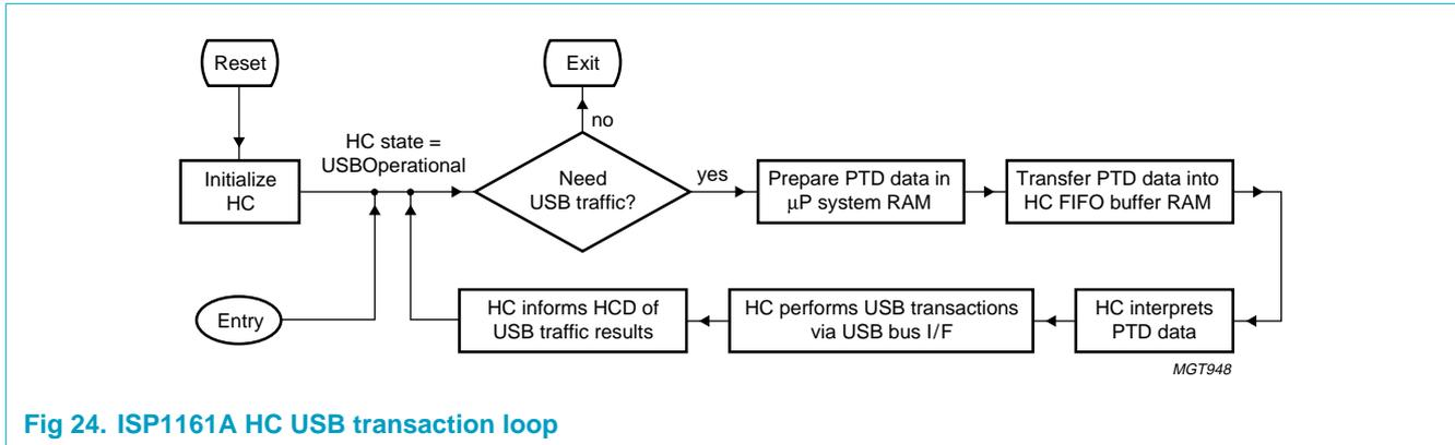
Fig 24. ISP1161A HC USB transaction loop
