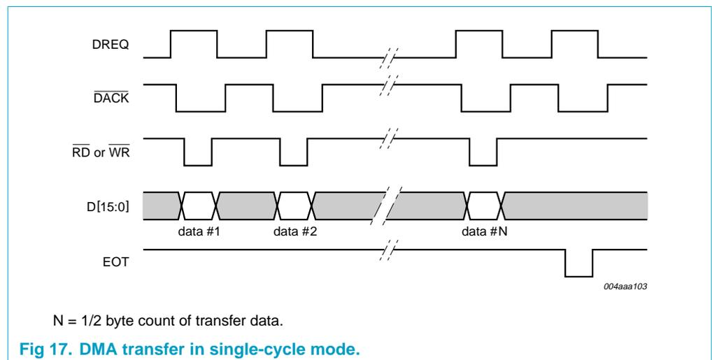
**Fig 17. DMA transfer in single-cycle mode.**
