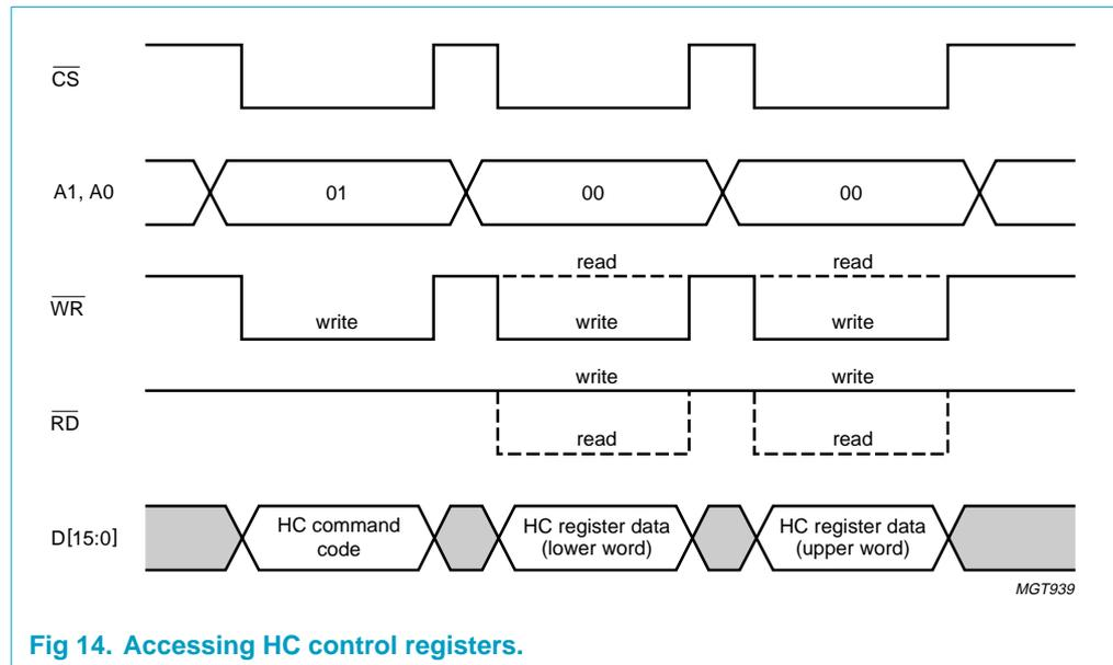
Fig 14. Accessing HC control registers.
