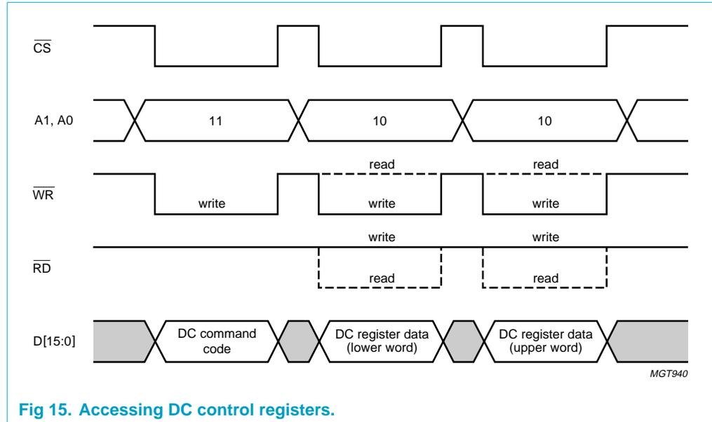
Fig 15. Accessing DC control registers.
