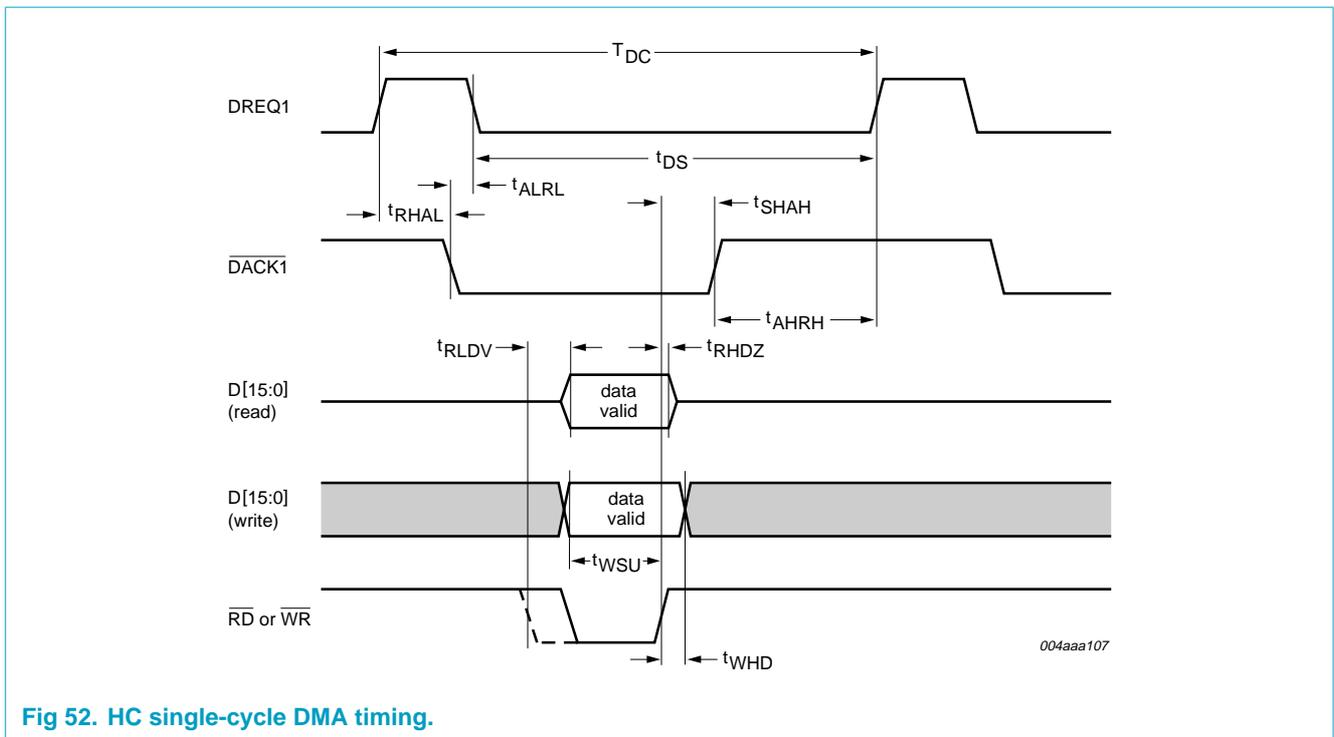
Fig 52. HC single-cycle DMA timing.
