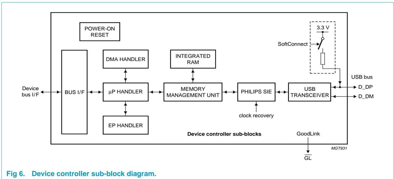
Fig 6. Device controller sub-block diagram.
