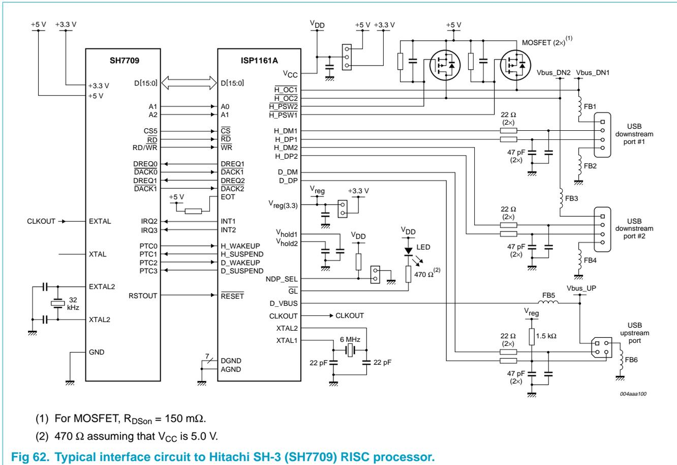
Fig 62. Typical interface circuit to Hitachi SH-3 (SH7709) RISC processor.
