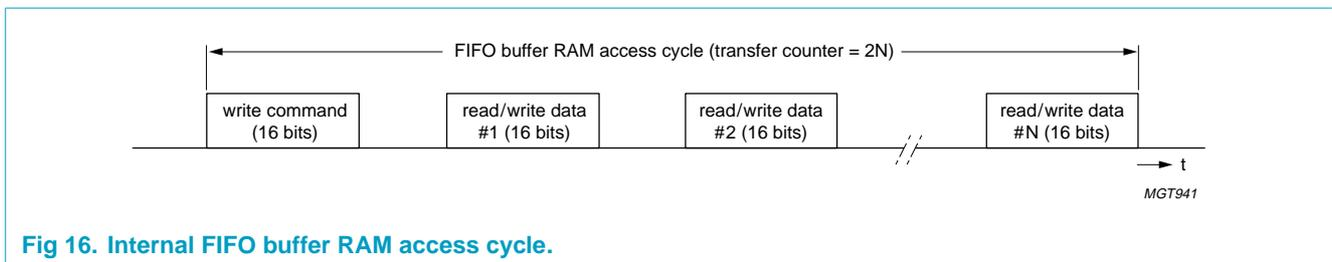
Fig 16. Internal FIFO buffer RAM access cycle.
