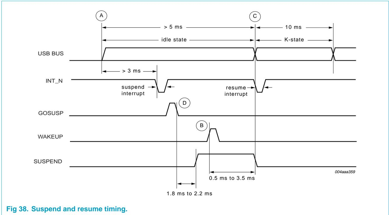
Fig 38. Suspend and resume timing.
