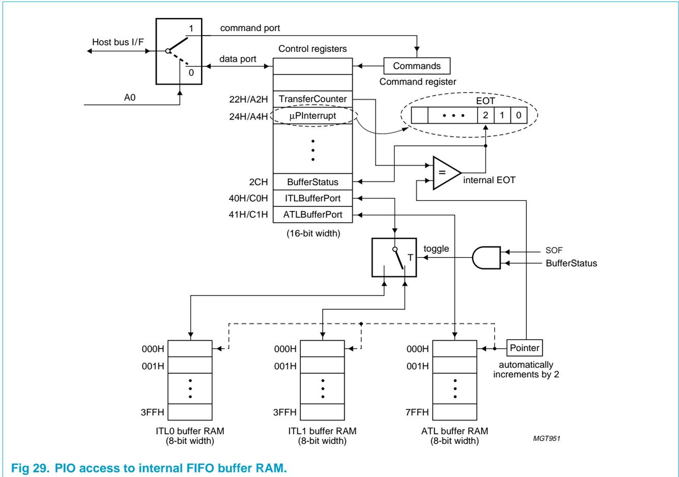
Fig 29. PIO access to internal FIFO buffer RAM.
