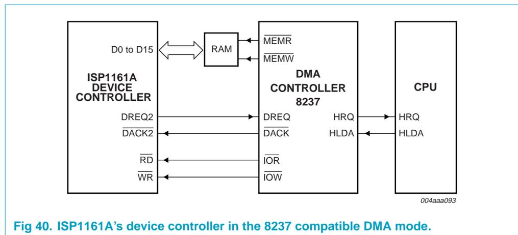
Fig 40. ISP1161A's device controller in the 8237 compatible DMA mode.
