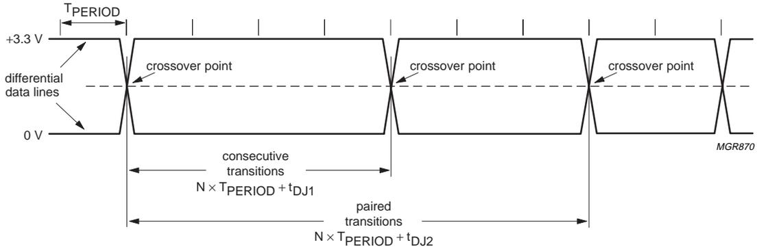
$T_{PERIOD}$  is the bit duration corresponding with the USB data rate.
