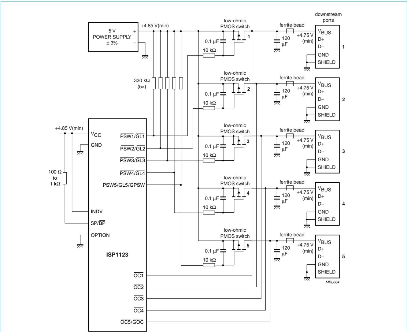
Power switches 1 to 5 are low-ohmic PMOS devices as specified in Section 13.2.
