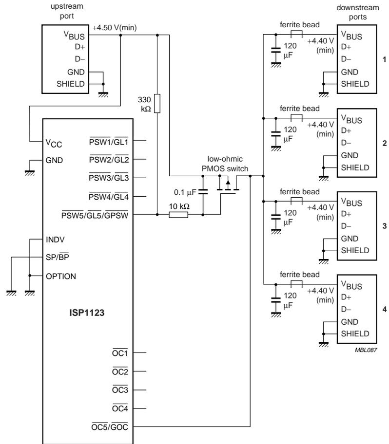
Power switch is low-ohmic PMOS device as specified in Section 13.2.
