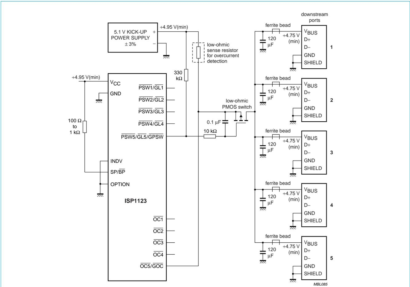
Power switch is low-ohmic PMOS device as specified in [Section 13.2](#).
