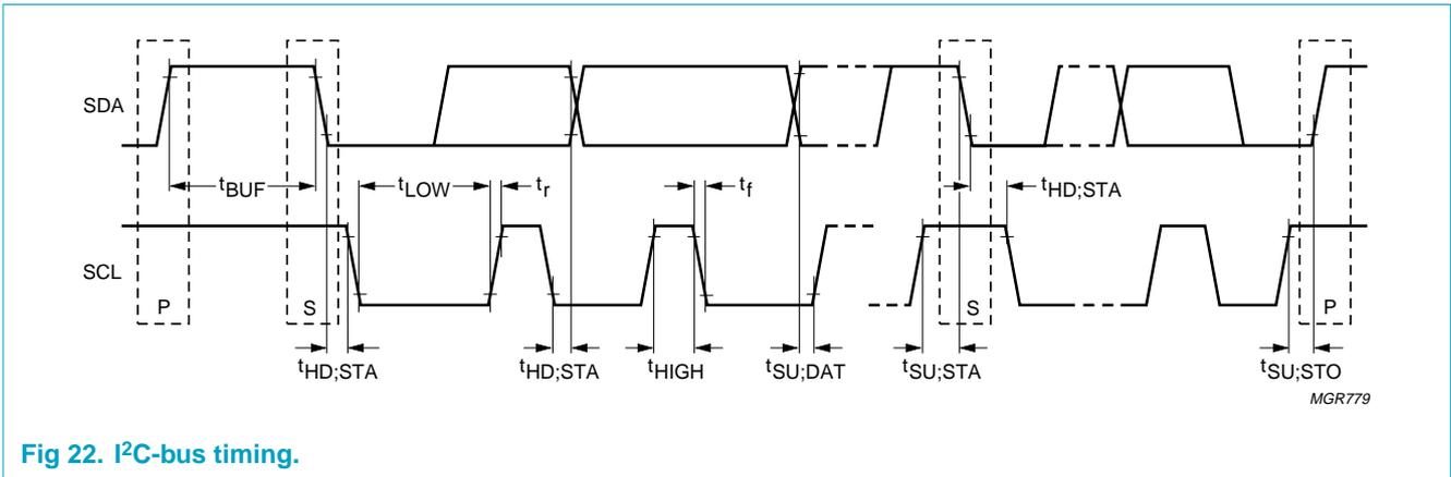
Fig 22. I<sup>2</sup>C-bus timing.
