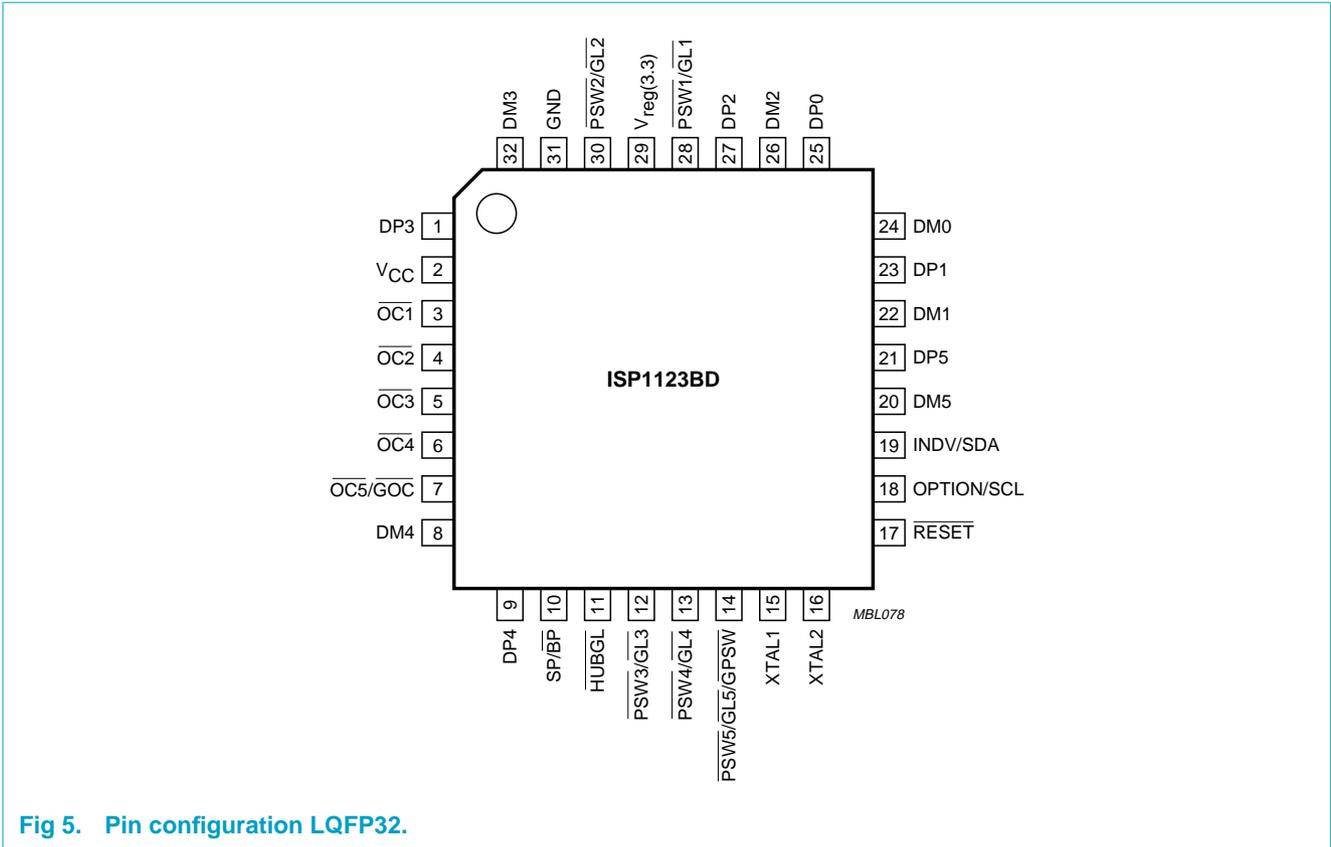
Fig 5. Pin configuration LQFP32.
