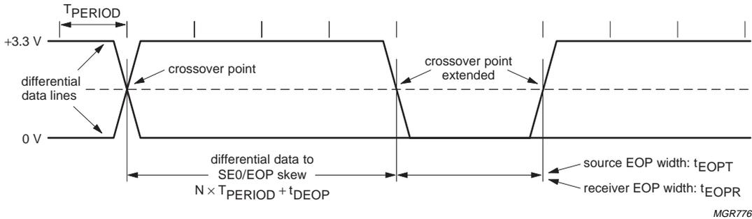
$T_{PERIOD}$  is the bit duration corresponding with the USB data rate.
