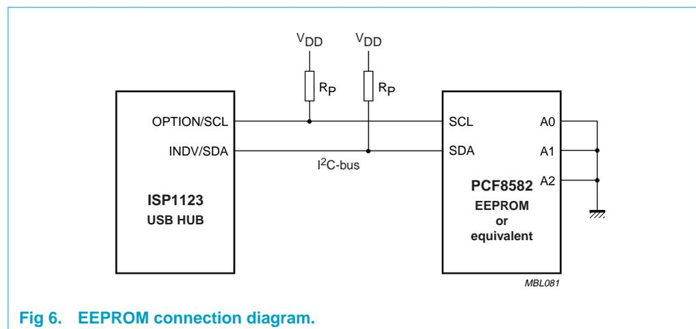
Fig 6. EEPROM connection diagram.
