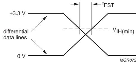
Fig 19. Receiver SE0 width tolerance.
