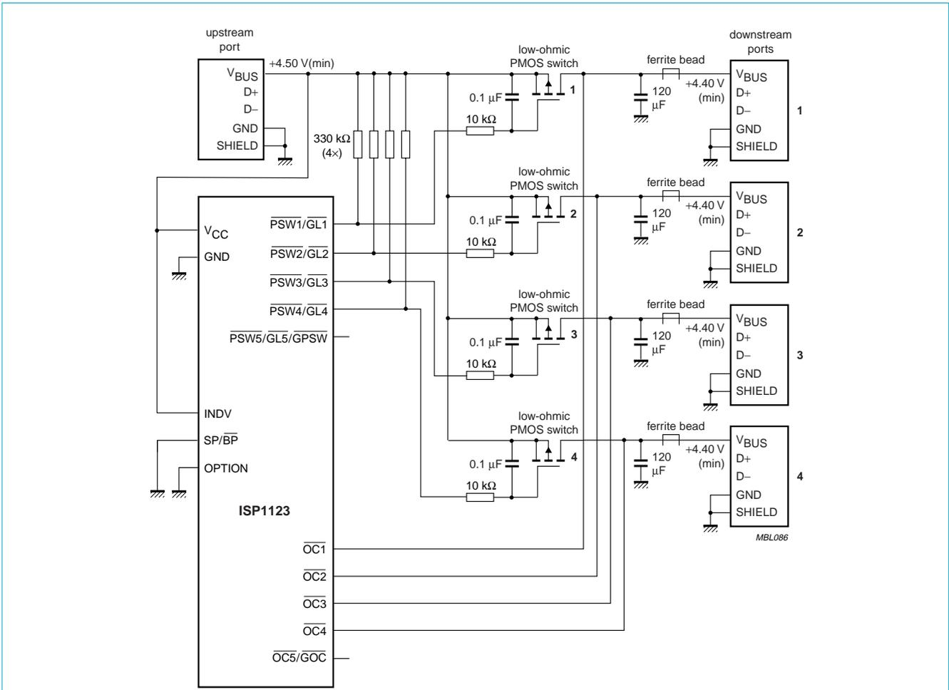
Power switches 1 to 4 are low-ohmic PMOS devices as specified in [Section 13.2](#).
