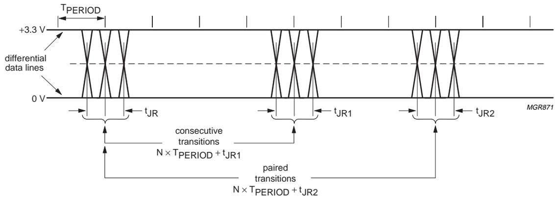
$T_{PERIOD}$  is the bit duration corresponding with the USB data rate.
