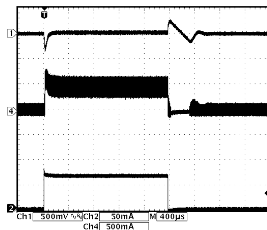
FIGURE 14. TRANSIENT RESPONSE ( V_{IN} = 3.3V ; V_{OUT} = 18.3V ; STEP LOAD CURRENT FROM 2.6mA TO 70mA)
