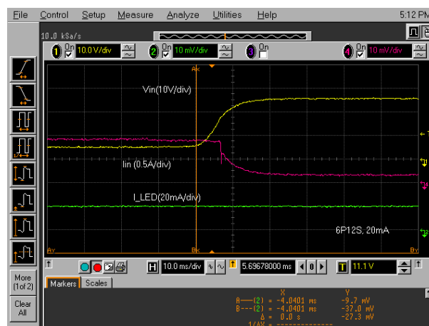
FIGURE 15. LINE REGULATION WITH V_{IN} CHANGE FROM 6V TO 26V, V_{IN} = 12V , 6P12S AT 20mA/CHANNEL
