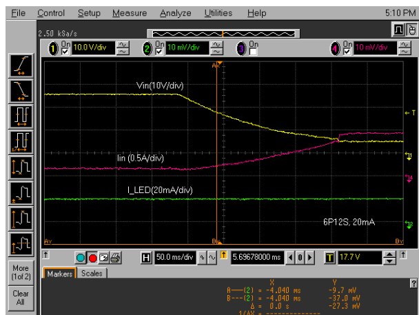
FIGURE 16. LINE REGULATION WITH V_{IN} CHANGE FROM 26V TO 6V FOR 6P12S AT 20mA/CHANNEL
