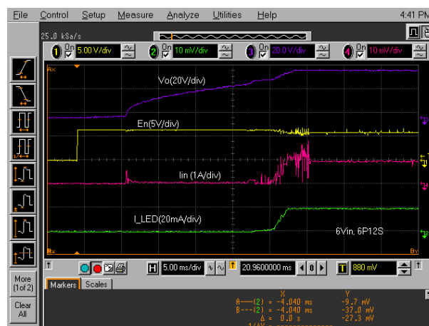
FIGURE 13. IN-RUSH AND LED CURRENT AT V_{IN} = 6V FOR 6P12S AT 20mA/CHANNEL
