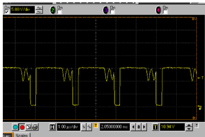
FIGURE 7. BOOST SWITCH NODE AT 100mA (PARTIAL DISCONTINUOUS)
