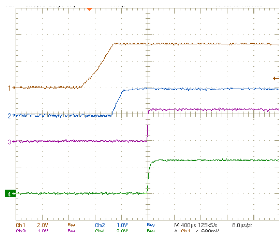
FIGURE 14. 4-CHANNEL DEFAULT START-UP @ NO LOAD CH1: VODCD1 (2V/DIV), CH2: VODCD2 (1V/DIV), CH3: VOLD01 (1V/DIV), CH4: VOLD02 (2V/DIV)
