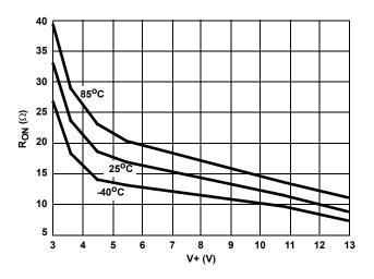
FIGURE 9. ON RESISTANCE vs SUPPLY VOLTAGE
