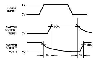
FIGURE 3A. MEASUREMENT POINTS (ISL84543 ONLY)
