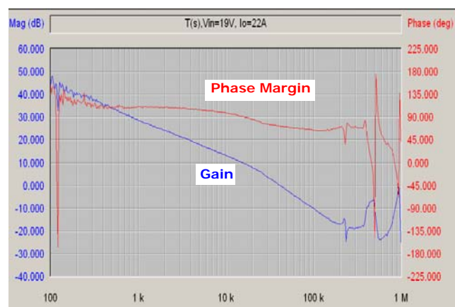
FIGURE 38. GPU MODE REFERENCE DESIGN LOOP GAIN T2(s) MEASUREMENT RESULT
