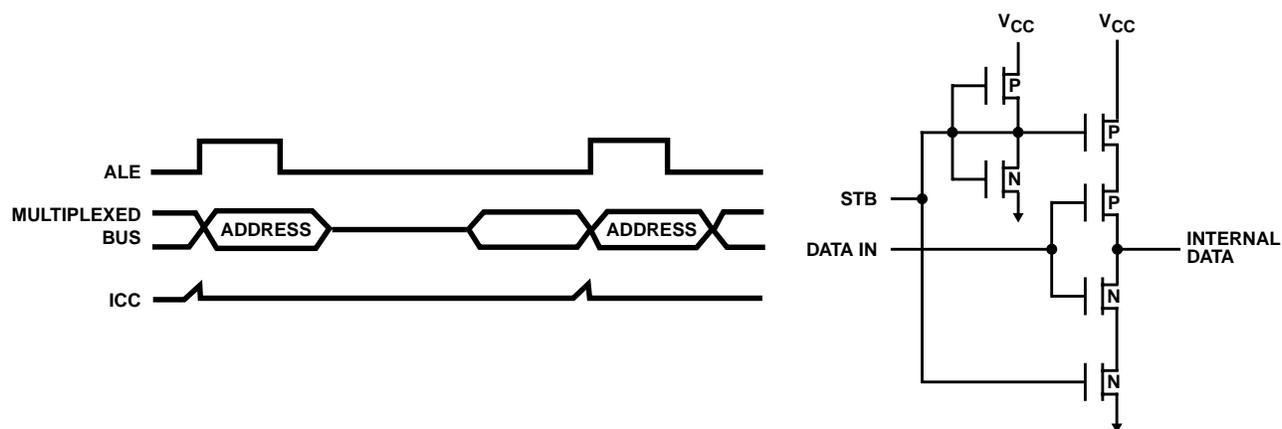
FIGURE 18. SYSTEM EFFECTS OF GATED INPUTS
