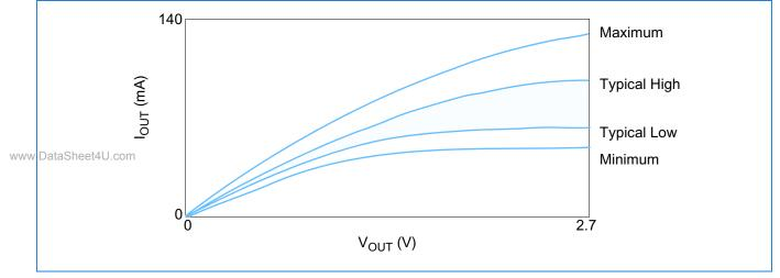
3. The full variation in driver pullup current from minimum to maximum process, temperature and voltage will lie within the outer bounding lines of the V-I curve.
