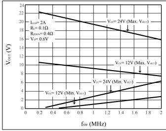
Figure 32 Minimum and Maximum Output Voltage versus Operating Frequency (minimum t<sub>ON</sub> and t<sub>OFF</sub> = 150ns)
