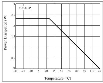
Figure 35 Dissipation Curve
