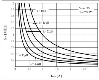
Figure 34 Inductance Selection Based On 30% Current Ripple
