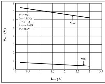
Figure 33 Minimum and Maximum Output Voltage versus LED Current (minimum t<sub>ON</sub> and t<sub>OFF</sub> = 150ns)
