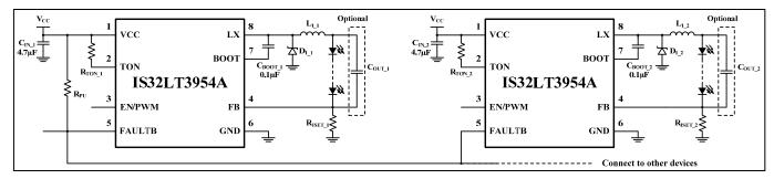
Figure 2 Typical Application Circuit (Several Devices In Parallel with FAULTB Interconnection)
