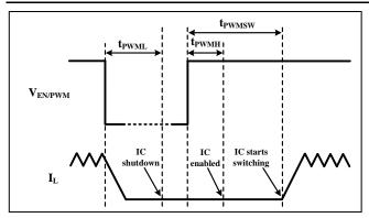
Figure 28 Device shutdown and enable
