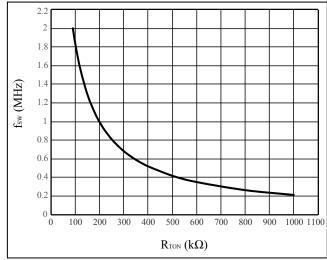
Figure 30 Operating Frequency vs. R<sub>TON</sub> Resistance
