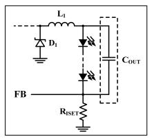
Figure 29 Adding Output Capacitor
