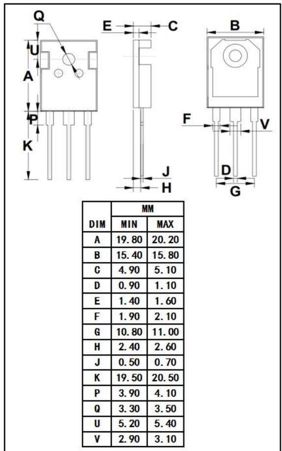
**isc N-Channel MOSFET Transistor****IRFP460A****ELECTRICAL CHARACTERISTICS**T<sub>C</sub>=25°C unless otherwise specified
