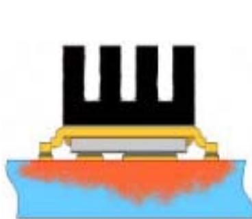
⑩ Mounted on minimum footprint full size board with metalized back and with small clip heatsink. (still air)
