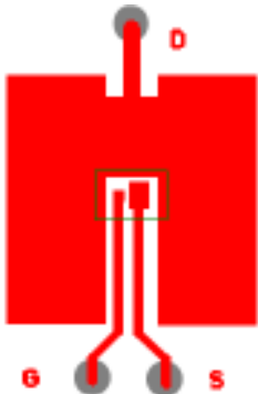
③ Surface mounted on 1 in. square Cu board (still air).
