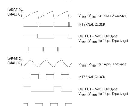
Oscillator timing capacitor  $C_T$  is charged by  $V_{REF}$   $t_c \approx 0.55 R_T C_T$ through R<sub>T</sub> and discharged by an internal current source. During the discharge time, the internal clock signal blanks the output to the low state. Selection of  $R_{\mathsf{T}}$  and  $C_{\mathsf{T}}$  therefore determines both oscillator frequency and Resultant frequency f =maximum duty cycle. Charge and discharge times are determined by the formulae:
