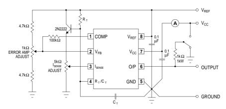
High peak current associated with capacitive loads necessitate careful grounding techniques. Timing and bypass capacitors should be connected close to pin 5 in a single point ground. The transistor and 5K potentiometer are used to sample the oscillator wave form and apply an adjustable ramp to pin 3.
