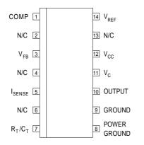
D-14 Package - 14 Pin Plastic (150) SOIC
