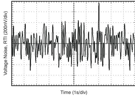
**Figure 6-14. INA282-Q1 0.1-Hz to 10-Hz Voltage Noise, RTI**
