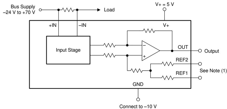
A. Connect the REF pins as desired; however, they cannot exceed 9 V greater than the GND pin voltage.
