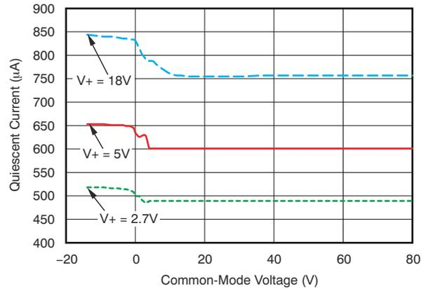
**Figure 6-8. INA283-Q1 Quiescent Current vs Common-Mode Voltage**
