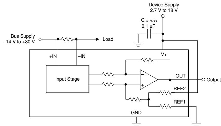
Figure 8-1. Basic Connections
