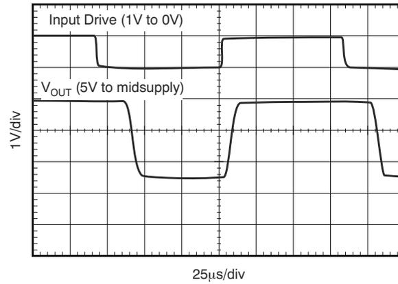
**Figure 6-31. Input Overload**
