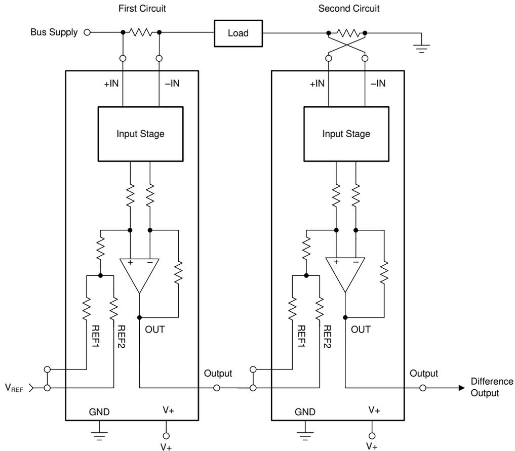
NOTE: The voltage applied to the reference inputs must not exceed 9 V.
