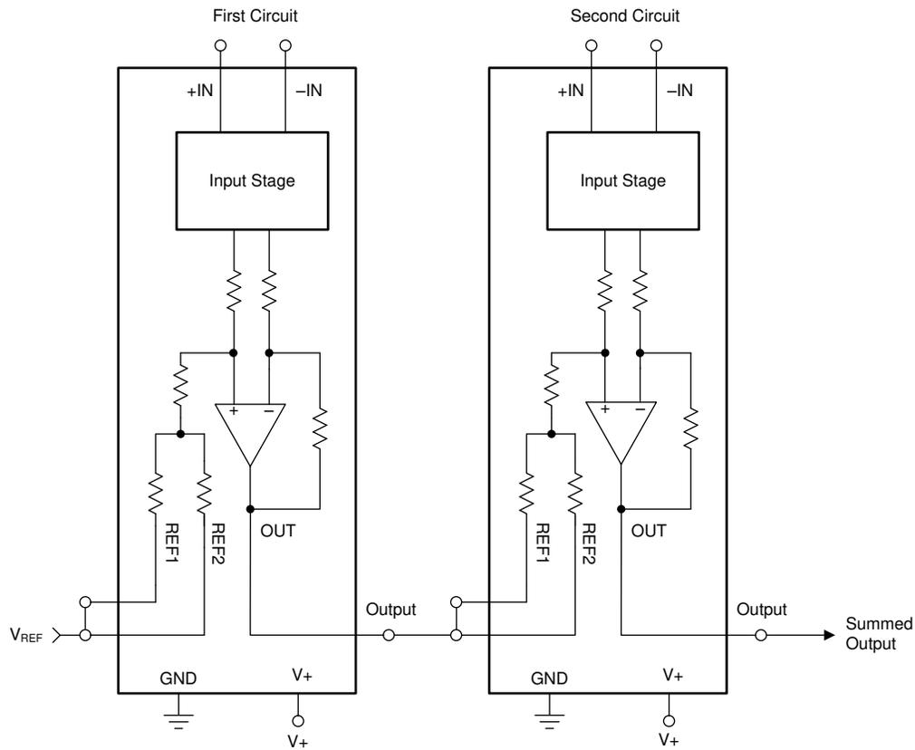
NOTE: The voltage applied to the reference inputs must not exceed 9 V.
