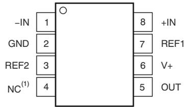
A. NC: This pin is not internally connected. The NC pin should either be left floating or connected to GND.
