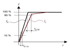
$t_{D,10}$  (delay time @ 10 %) and  $t_{D,90}$  (delay time @ 90 %)
