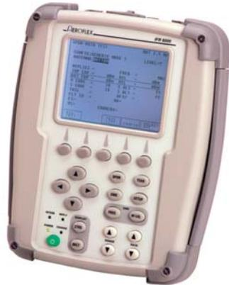
The IFR 6015 is a compact, lightweight and weatherproof unit designed for testing transponder modes A/C/S, TCAS I, II and Military E-TCAS as well as DME.
